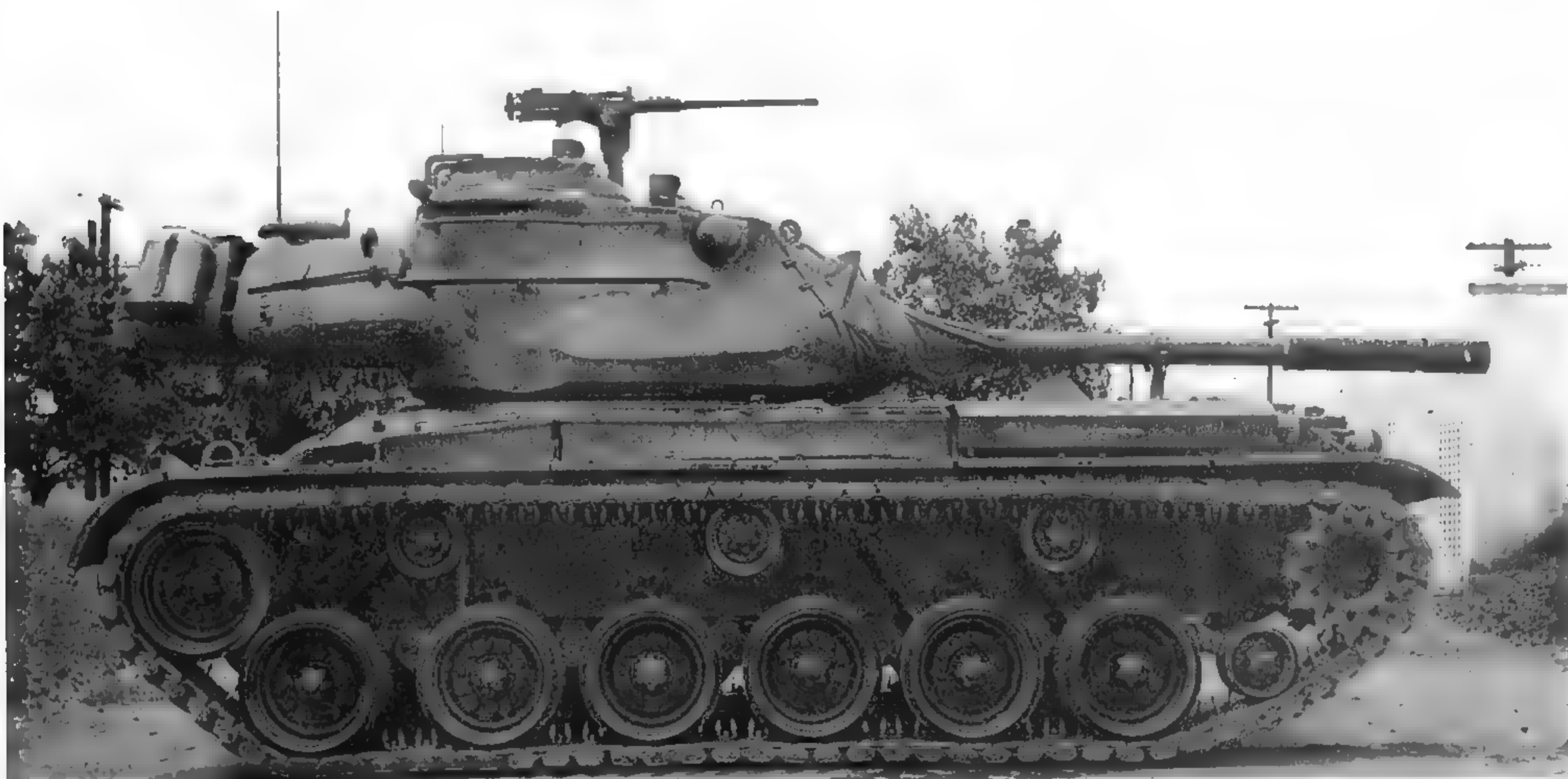
This M47 is shown minus its sand shields over the return track, and with the main gun in the travel position. (Photo courtesy of Patton Museum)
